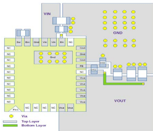
Figure 6: Recommended PCB Layout
